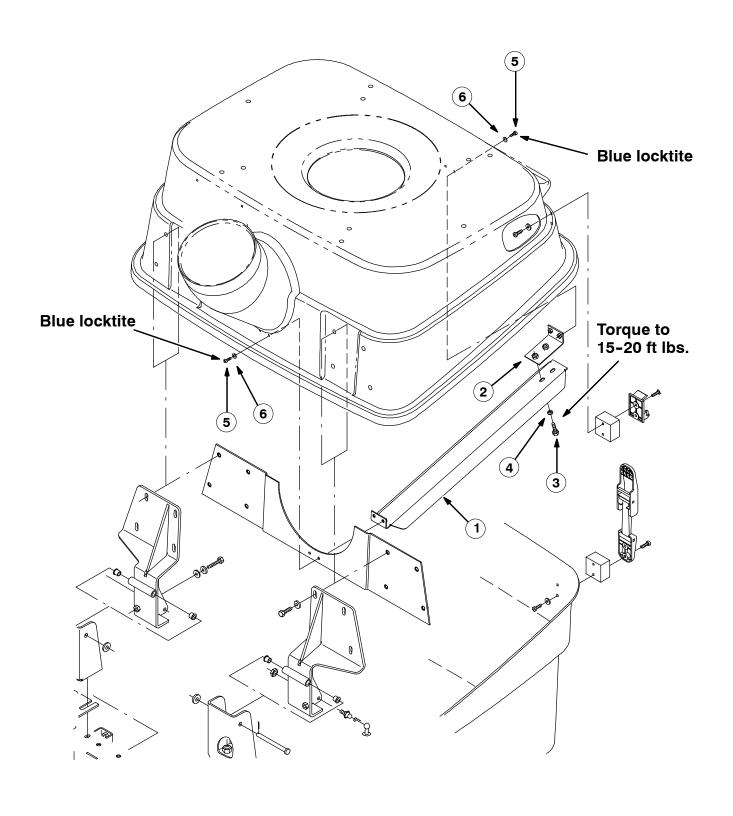
FIG. 1 - INSTALLATION, PLENUM BRACE KIT 368105
